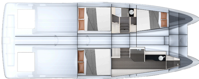
The Voyage solution, where one hull houses a single cabin, one two doubles. In the case of the Holiday version, both hulls accommodate two doubles as is the case here in the case of the left hull
