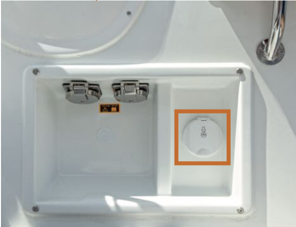
Located on starboard transom, fresh water pump is connected to starboard fresh water standard tank.
