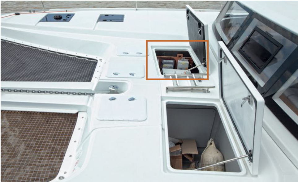
[Forward starboard technical compartment]
