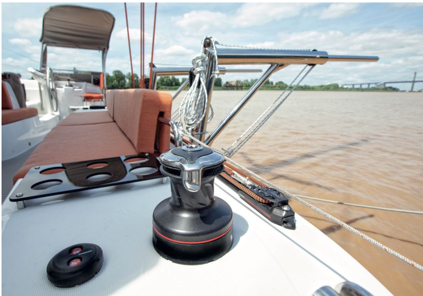
Electrical upgrade for manual winch for davits [portside]
