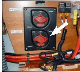
CUT-OUT PORT ENGINE
