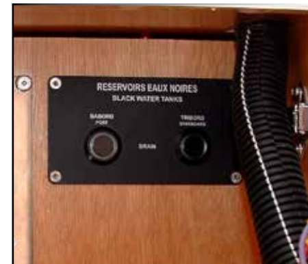
BLACK WATER TANK DRAIN SWITCHES
