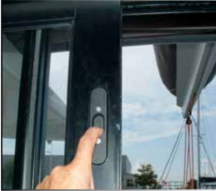
EXTERNAL BLOCKING SYSTEM FOR THE ENTRANCE DOOR
