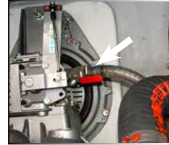
ENGINE WATER INTAKE VALVE
