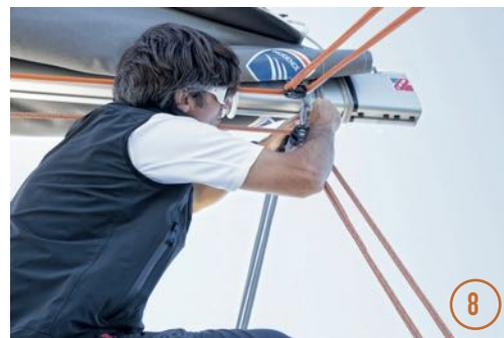
On EXCESS 11 you can cleat it to the aft mooring cleats, on starboard if you are on a port tack, or on port if on a starboard tack. You will balance the tension on the flying barber-hauler and the leeward mainsheet to get a proper shape.
