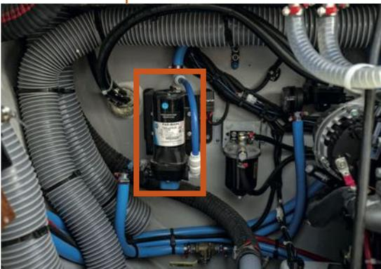
ON/OFF switch on water pump is located in port engine compartment.
