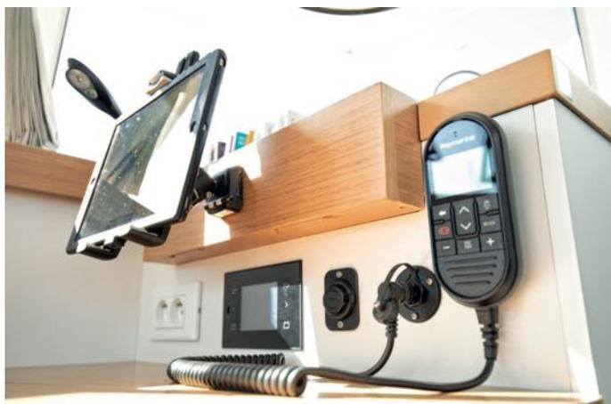
VHF Ray90 ASN combined with active speaker [Raymarine model: A80543] and wireless station [Raymarine model: A80540].
