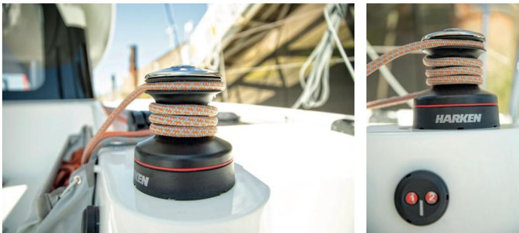
Electric upgrade from manual winch [per standard] on **starboard** helm station.
