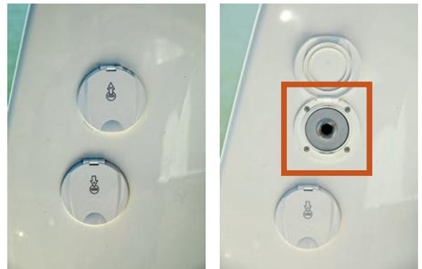
Located on port transom, fresh water pump connected to fresh water standard tank.
