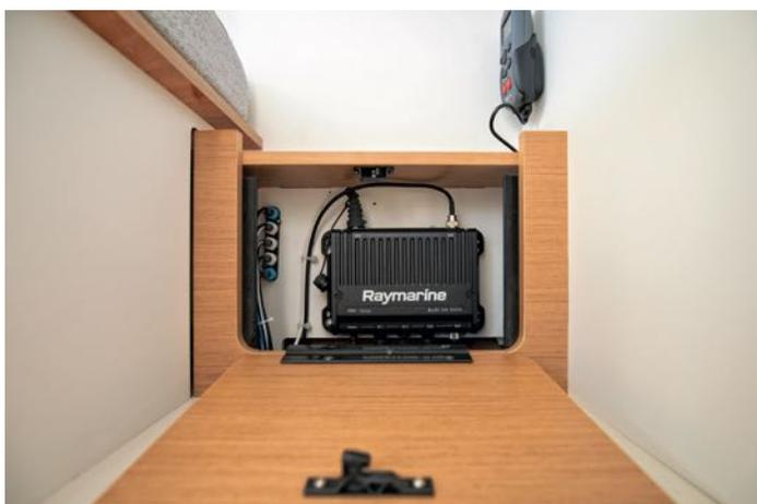
**AIS 700 Class B Transceiver** with integrated antenna splitter [Model: E70476]
