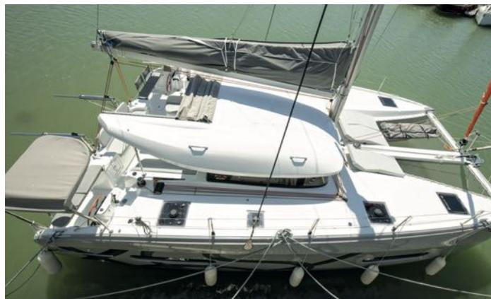
Manual sliding roof. Replaces the standard GRP roof.
