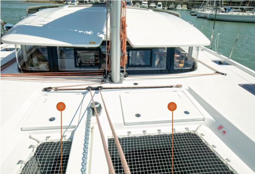
An additional fresh water tank is available on starboard [300 L | 79 US gal].
