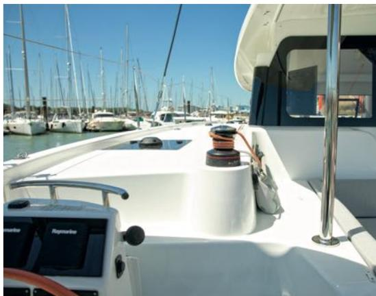
Electric upgrade from manual winch [per standard] on **port** helm station.
