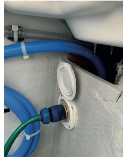
A manual valve and the inlet, are located in the port forward deck locker. The valve allows the selection between sea water and fresh water.
