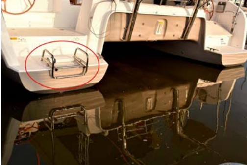
Reboarding device: Swimming ladder (Ref 1):
