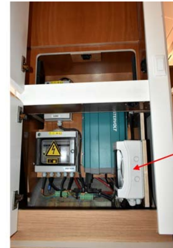
Ref 3: Differential switch (Operation) Location: Starboard aft cabin
