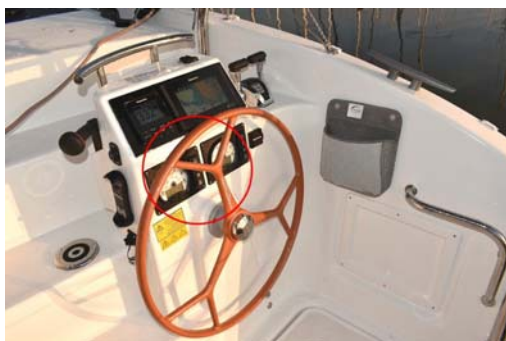
Engine instrument panel Location: Cockpit
