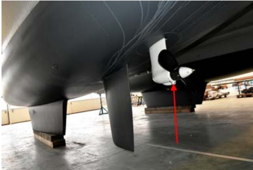
Engine base anode
