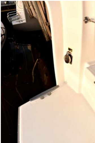
Ref 1: AC shore socket (onboard & Air conditioning) Location: Starboard cockpit
