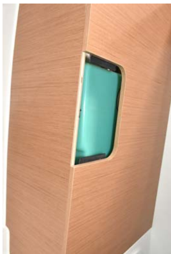
Blackwater tank Location: in each head
