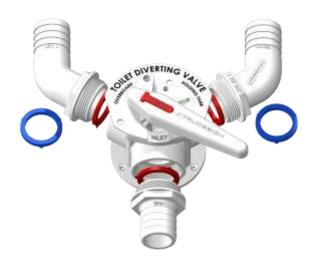
Legislation in many countries dictates the use of holding tanks near shore, or in defined areas. By installing a diverting valve (Y Valve), the user has the choice to divert black water to a holding tank or directly overboard when circumstances allow.
