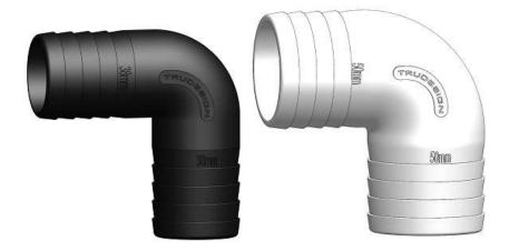
TruDesign Connectors are moulded from a glass reinforced nylon composite. High strength, high-modulus glass fibres impregnated into the nylon provides dramatic strength, stiffness, toughness, and dimensional stability. TruDesign Connectors eliminate the corrosion and electrical bonding problems associated with metallic fittings. The Connectors are designed for twin hose clamps, and to not crush under high load conditions.
