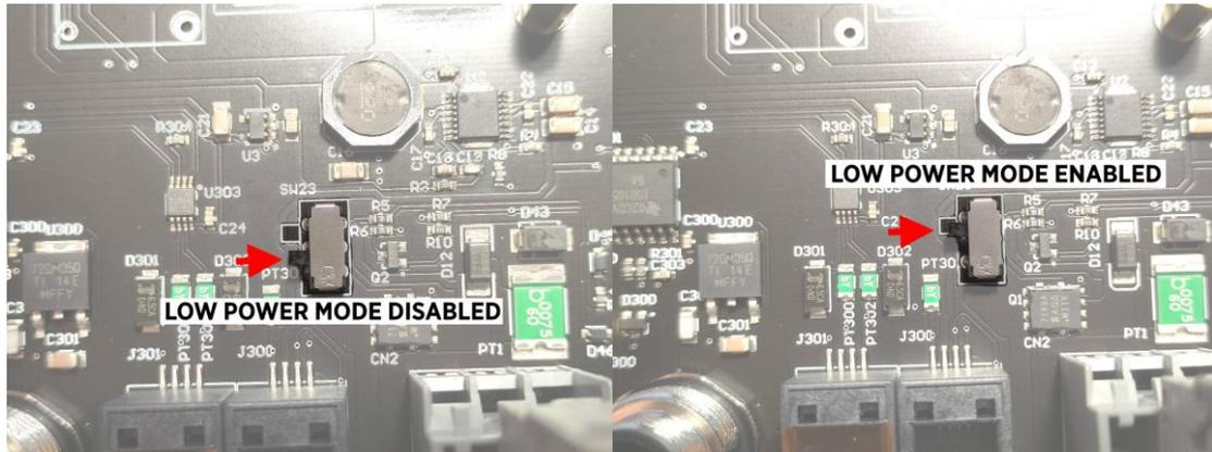
Figure 2: Low power mode enable/disable switch.
