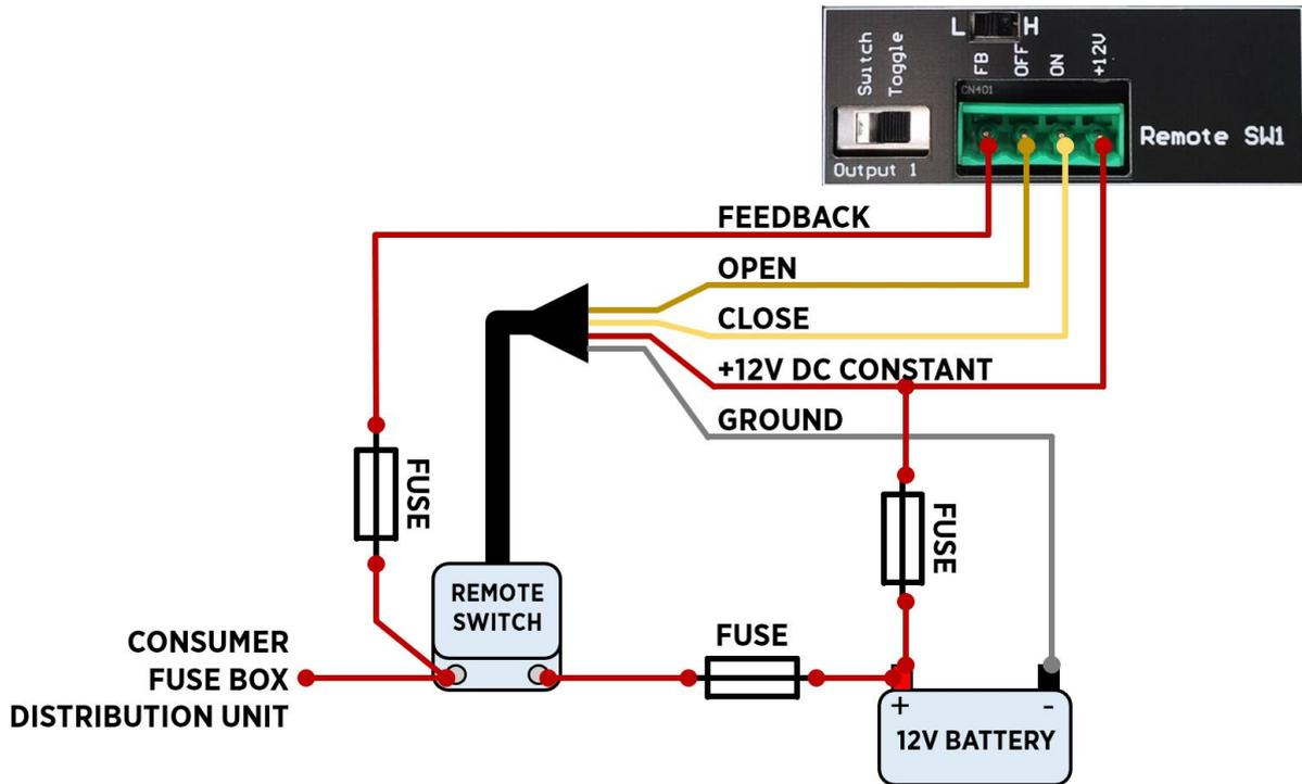
*Figure 10: Feedback signal from remote switch output.*
