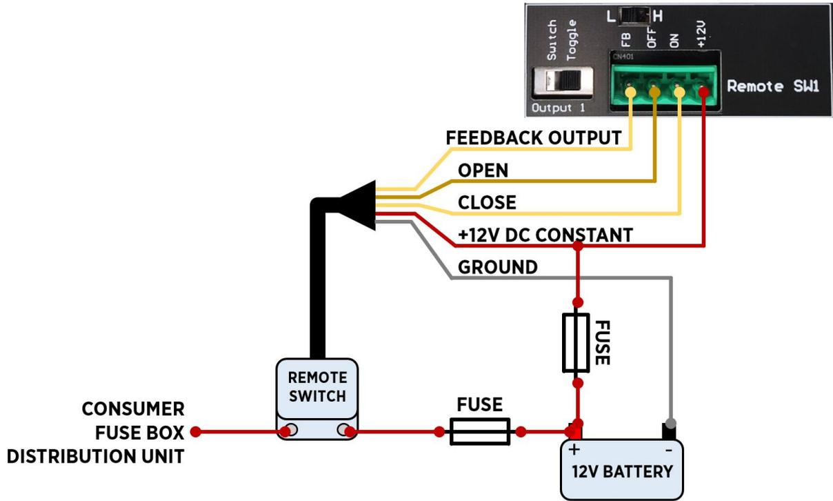
Figure 8: Toggle signal type of remote switch.
