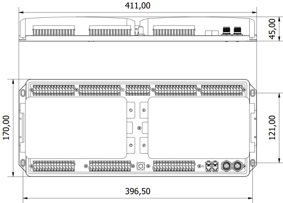
Figure 20: SPU303 DC Distribution Unit general dimensions.
