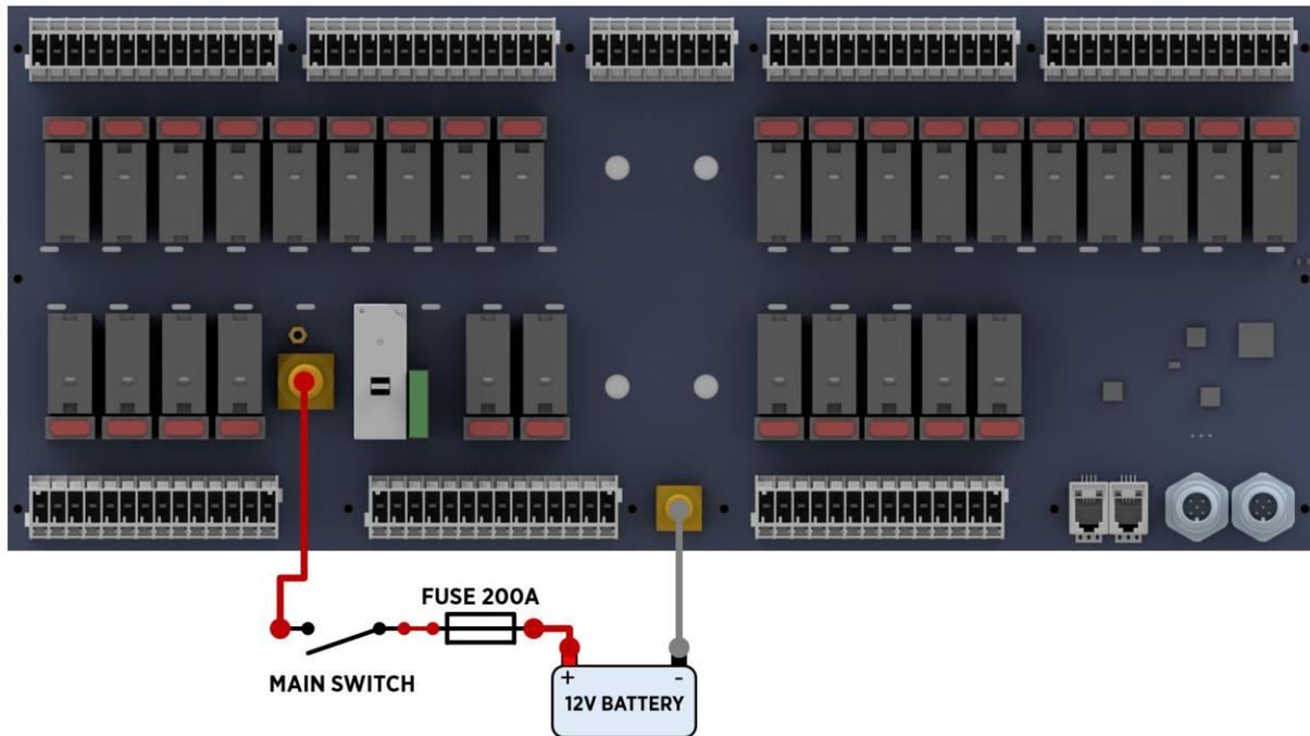
Figure 13: Power source for the DC distribution unit.
