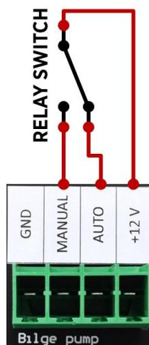
Figure 5: Internal schematics of the bilge pump connector.
