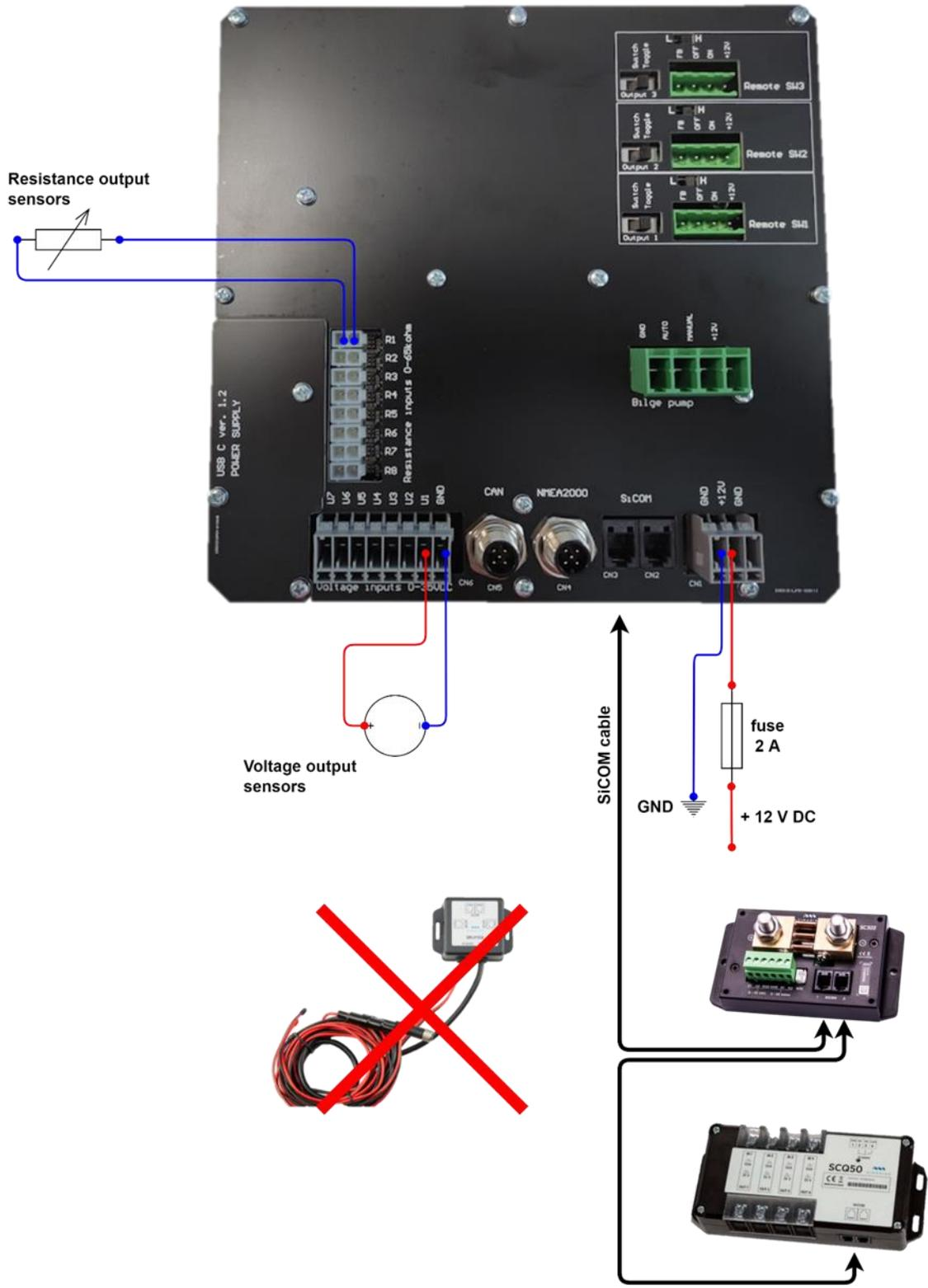
Figure 3: Control panel connections diagram.
