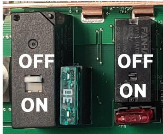
*Figure 15: Tabs on relays for manual switching.*
