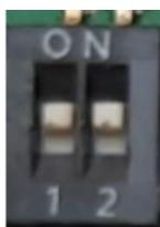
SW4 toggle switches positions to enable controlling both outputs with both buttons simultaneously.
