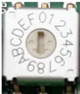
Each button can be set to work in multiway switching or not. This is established with proper position on SW6.
