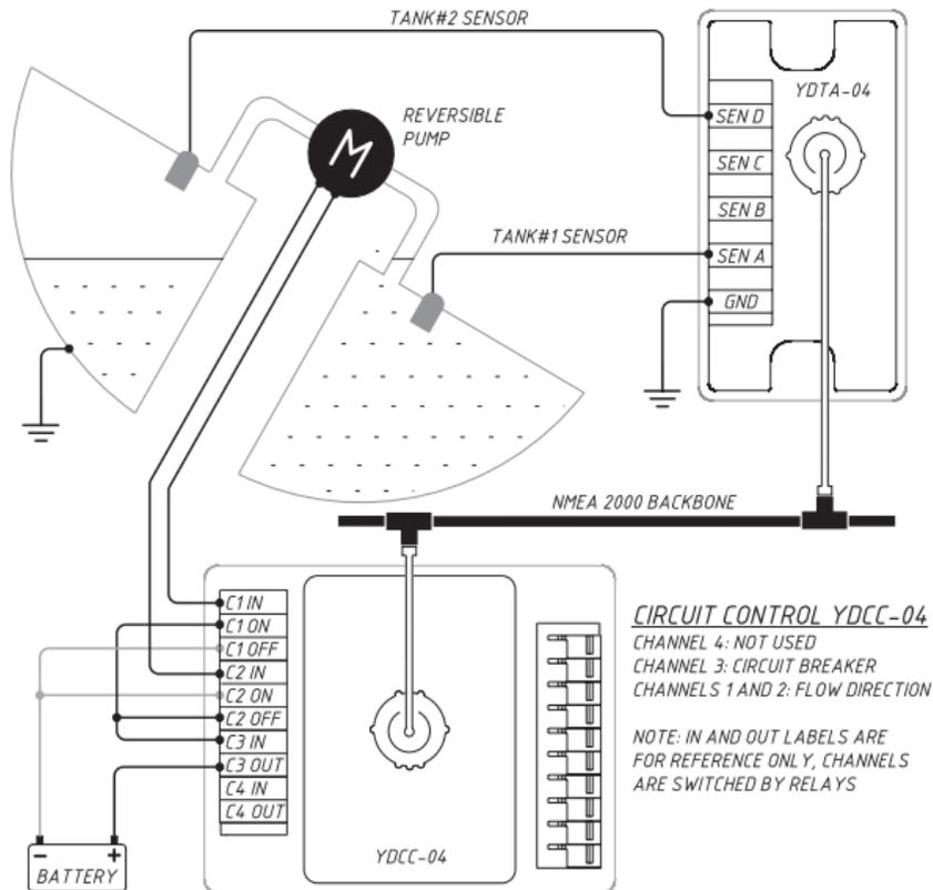
Figure 1. Automatic management of ballast tanks with YDCC-04 and YDTA-04
