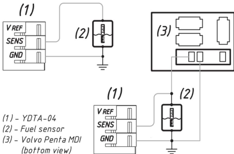
Figure 1. Standalone sensor connection (left) and connection in parallel with Volvo MDI unit (right)
