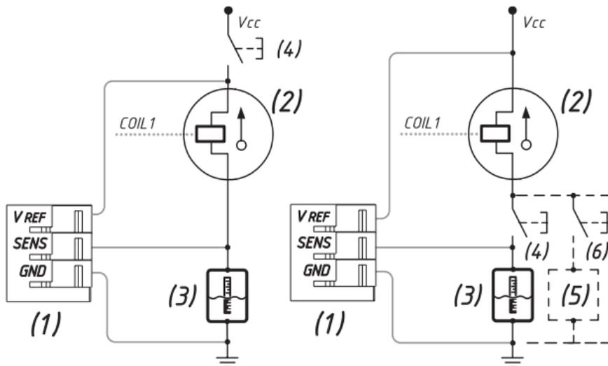
(1) – YDTA-04, (2) – Gauge, (3) – Fuel Sensor, (4) – Optional Button, (5) and (6) – Parallel Sensors (optional)
