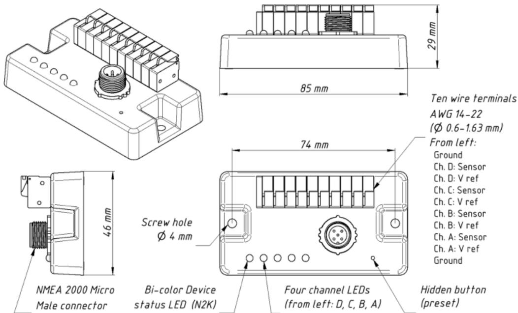
Figure 1. Drawing of Tank Adapter YDTA-04N
