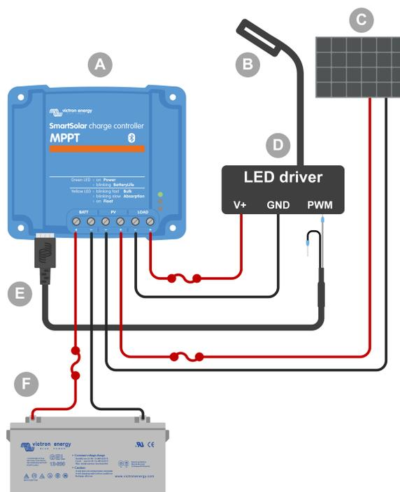
Wiring example - Controlling a streetlight LED driver.
