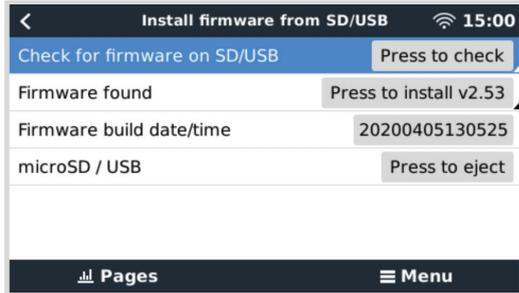
There may be reasons why it is necessary to manually download and install a specific firmware version (e.g. an older firmware version that is not stored under "Stored backup firmware" on the GX device). This chapter explains how to do that.
