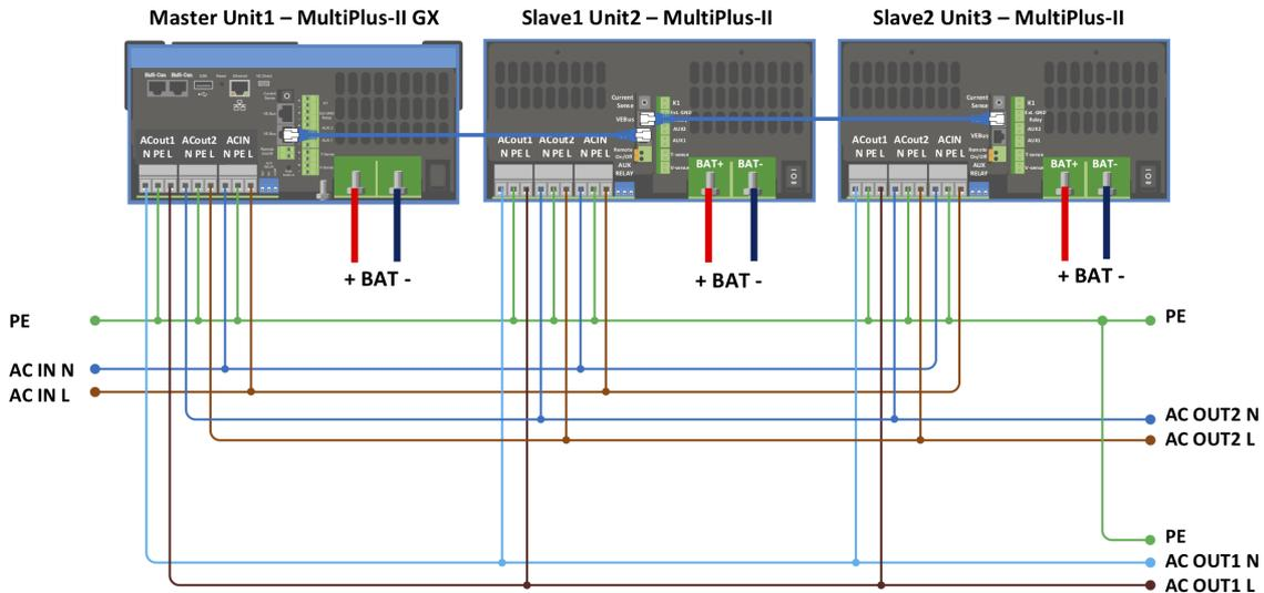
Additional conditions are required for parallel systems - please read further specific documentation here - [https://www.victronenergy.com/live/ve.bus:manual\\_parallel\\_and\\_three\\_phase\\_systems](https://www.victronenergy.com/live/ve.bus:manual_parallel_and_three_phase_systems)
