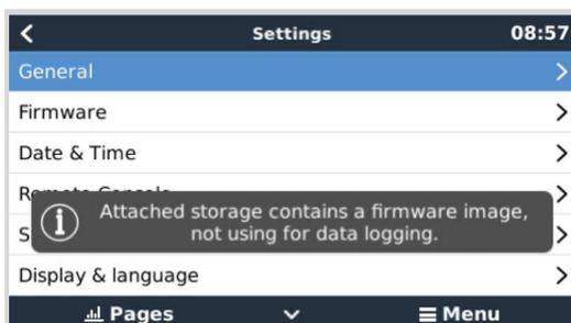
Note that you will see a warning “Attached storage contains a firmware image, not using for data logging.”. That warning can safely be ignored.
