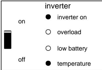
The inverter has switched off due to the electronics temperature being too high.
