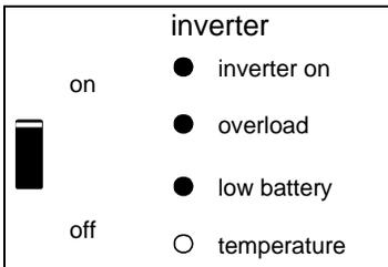
The inverter switched off due to excess ripple voltage on the battery terminals.
