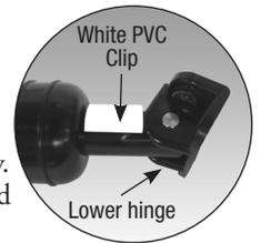
**Step 4 - Important:** Insert the sensor rod into the piston (see Figure 4). Make sure that the O-ring is in place inside the new upper hinge. Insert the upper hinge spacer (see Figure 4) into the inside of the cylinder (Flanged edge facing up). Screw the new upper hinge onto the cylinder while keeping the sensor rod inserted into center of the piston. Tighten the upper hinge as tight as you can by hand.
