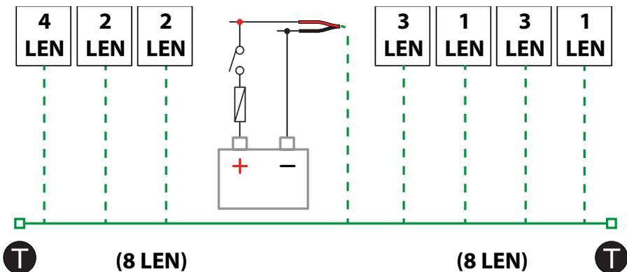
→ *Note: Do not connect the NMEA 2000® power cable to the same terminals as the engine start batteries, autopilot computer, bow thruster or other high current devices.*
