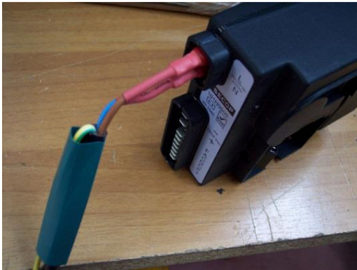
Figure 11: Detail of double insulated connection
