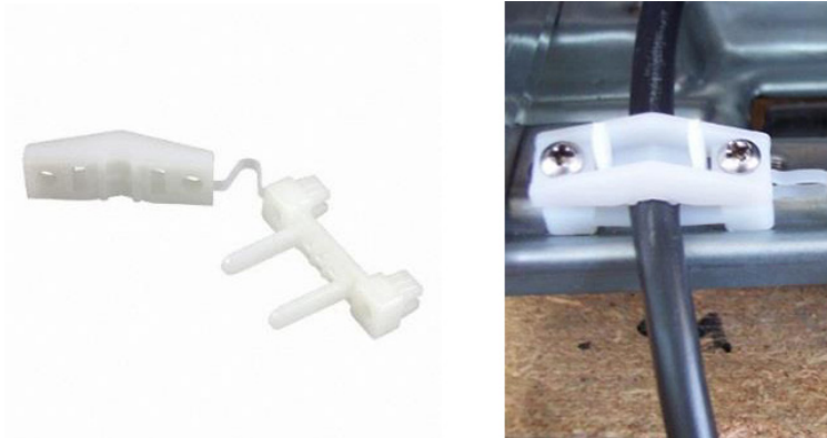
Figure 13: Detail of cable double fastening
