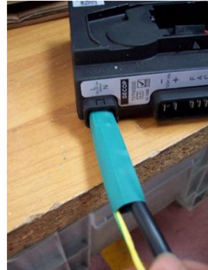
Figure 11: Detail of double insulated connection
