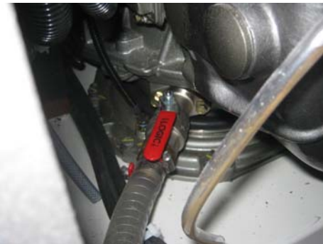
Engine water intake valve: Located directly on the saildrive
