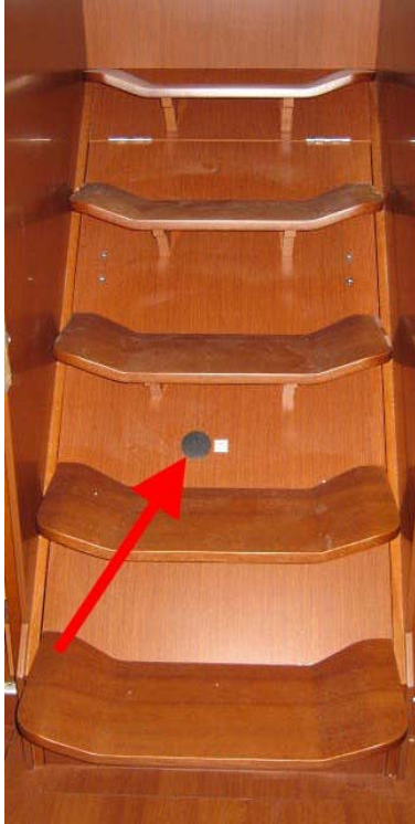
Location of the fire extinguisher port: Companionway
