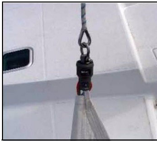
FIXING OF THE GENNAKER HALYARD ONTO THE HEAD
