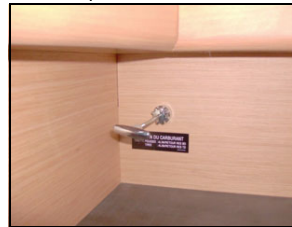
Lever pulled: Starboard tank
