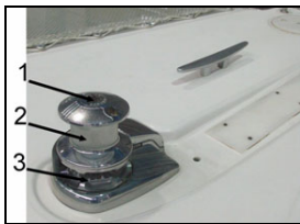
1 - Handle position (The handle is used to disengage the chain rim brake and to haul in the anchor manually in the case of electrical breakdown)
