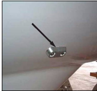
ANODE (On hull, under water line)
