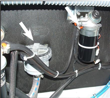
Inspect and clean the water filters regularly (access in the engine bilges).
