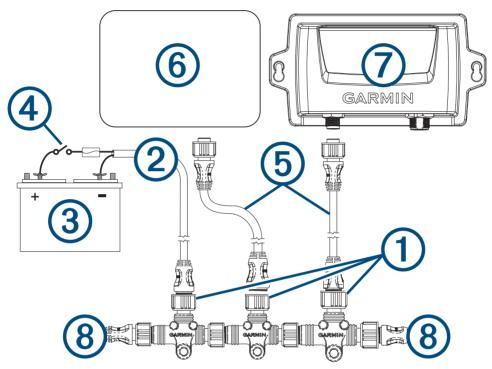
2 Connect the included NMEA 2000 power cable ② to a 9 to 12 Vdc power source ③ through a switch ④. You should connect the power cable to the ignition switch of the boat if possible, or route it through an inline switch (not included).
