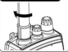
1. To install the antenna turn the antenna into the radio clockwise to tighten. Do not overtighten.
