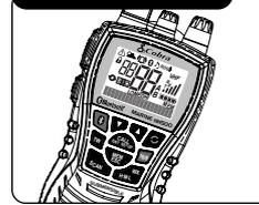
Refer to the foldout at the front of this manual to identify the various controls and indicators on your radio. Throughout this manual you will be instructed to “Press” or to “Press and Hold” various buttons (except “Push to Talk”) on the radio. “Press” means a momentary press of approximately one (1) second. “Press and Hold” means to hold the button down for approximately two (2) seconds.
