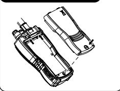
When your rechargeable batteries begin to discharge too quickly, it is time to install a new battery pack. Your radio will also operate with five (5) high-quality AA alkaline batteries, using the included alkaline battery tray.
