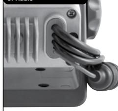
Cobra Positioning System Plug
