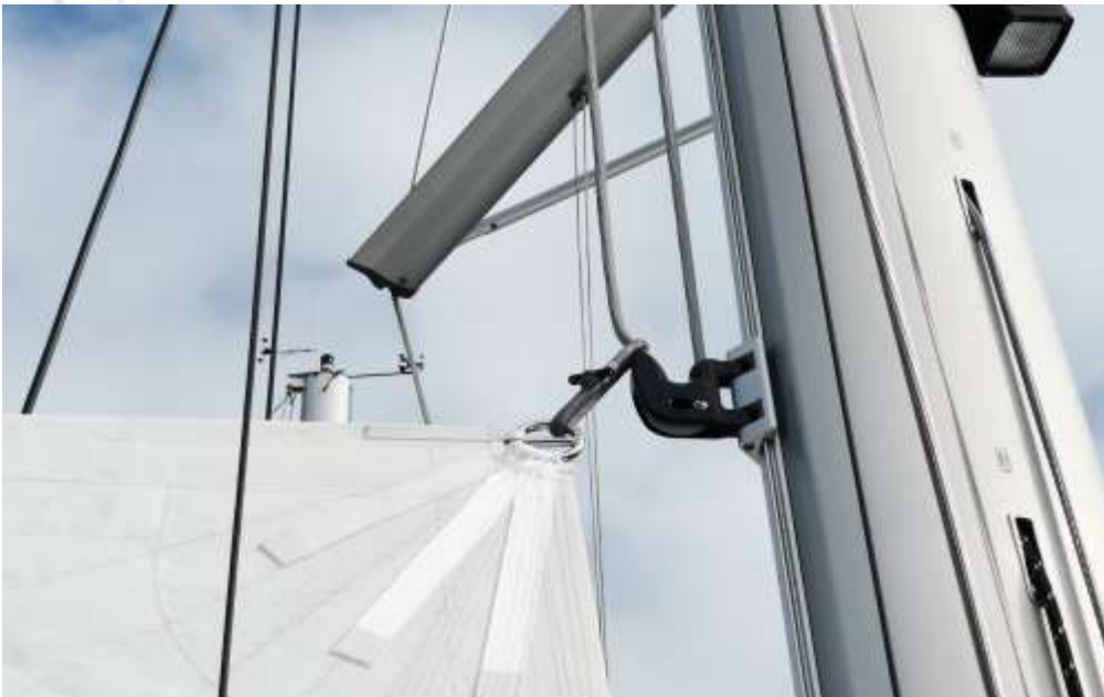
Pic 4. Loop not engaging hook.
