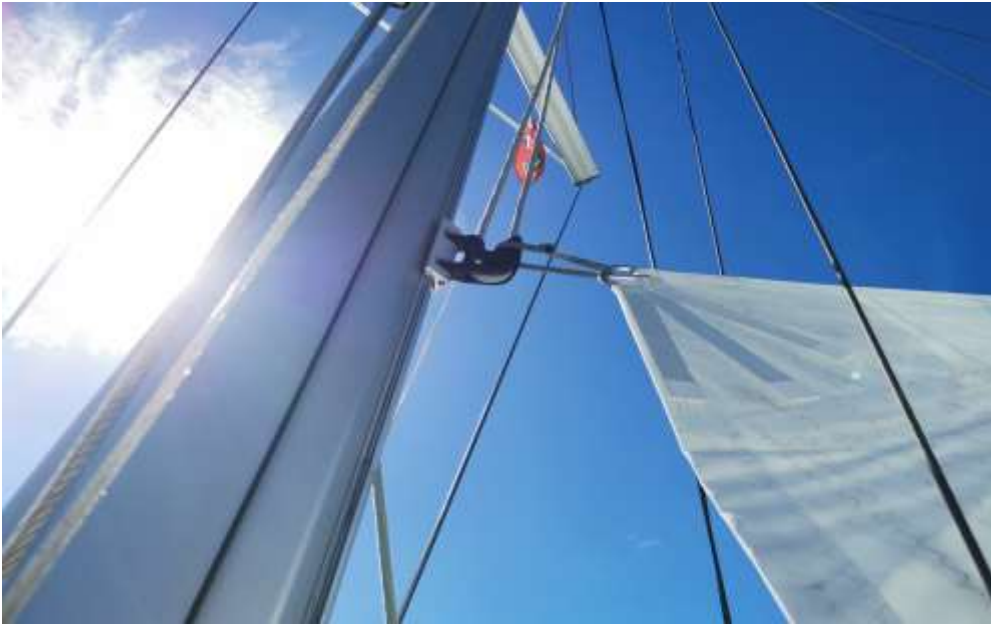
Pic 3. Looped line sitting on Halyard hook
