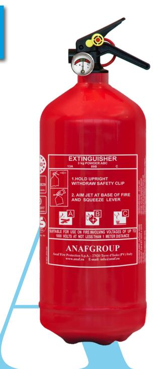
PS3-HX ABC is a stored pressure, multi-purpose dry powder fire extinguisher with pressure gauge. Wide operating temperature range –30 °C +60 °C, ensuring suitablility for use in low-temperature countries.
