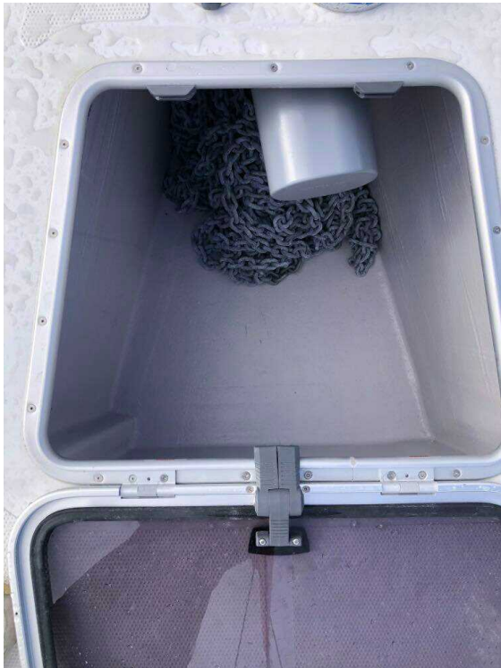
Deep anchor locker and access to bow thruster at the front of the central float
