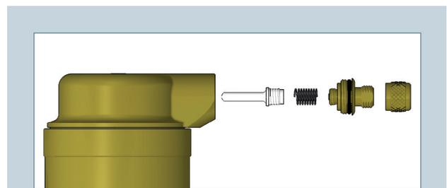
It is possible to rotate the air vent valve through 360° to position the drain appropriately, without needing to shut down the system.
