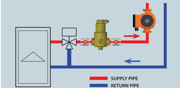
**!** In cooling systems the deaerator should be installed on the return pipe.
