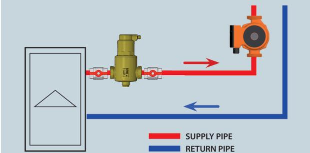
**CORRECT INSTALLATION IN SYSTEM WITH MIXING VALVE**
