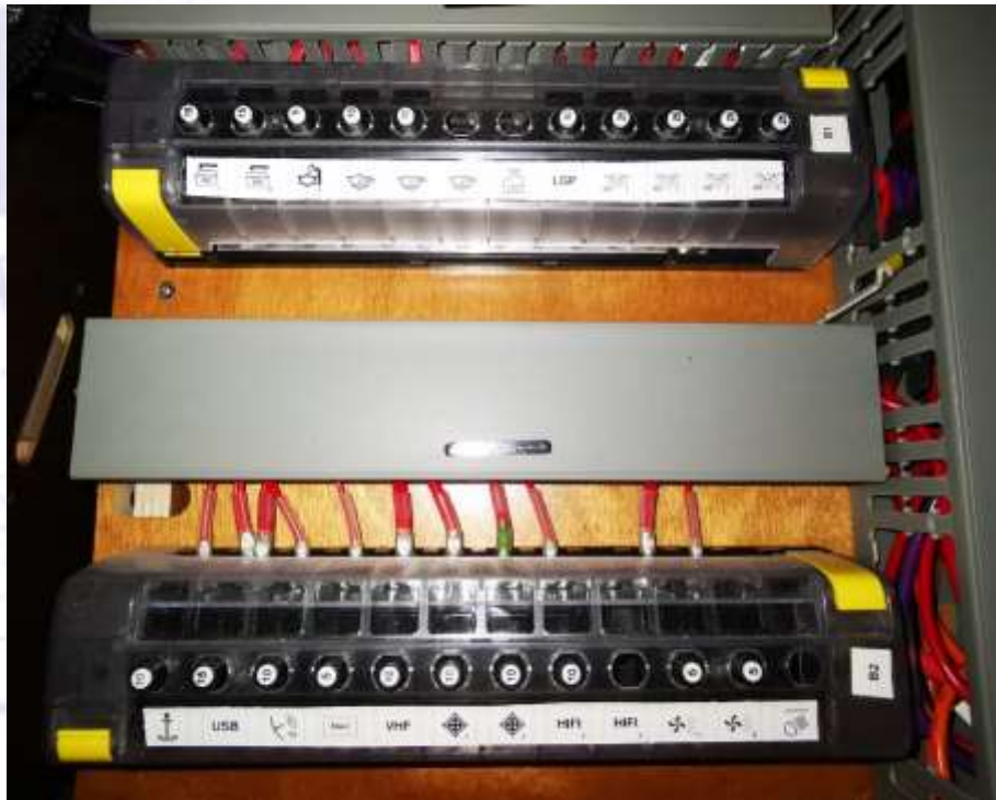
Fuses in starboard forward companion way locker
