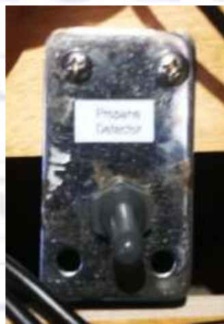
Propane detector switch behind starboard aft cabin door
