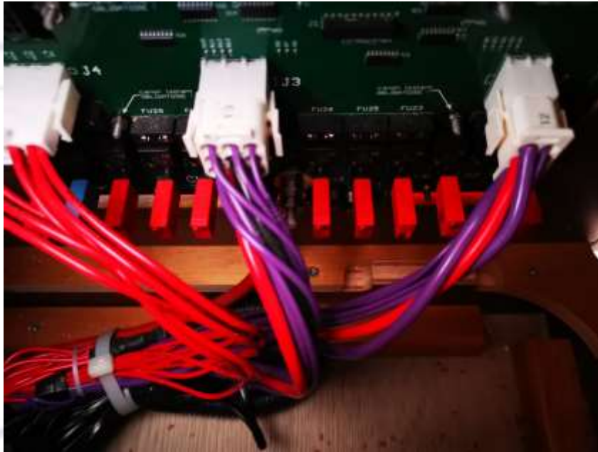
Fuses in starboard forward companion way locker
