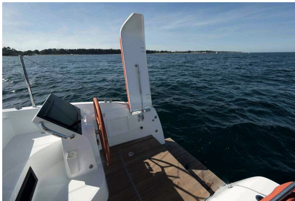
Double foldable seat on starboard helm station. New design: one-piece composite seat.
