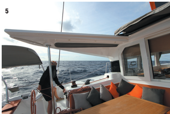
5/ The corners of the bimini mask the sailplan from the maneuvering positions: you need to lean outboard to see.
