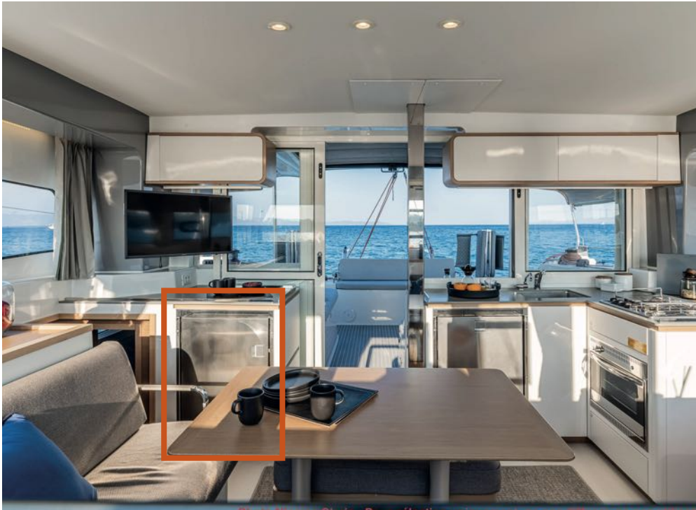
Additional 12V fridge [130 L | 34 US gal] on port galley. Replaces the storage unit per standard. [Not compatible with freezer option]
