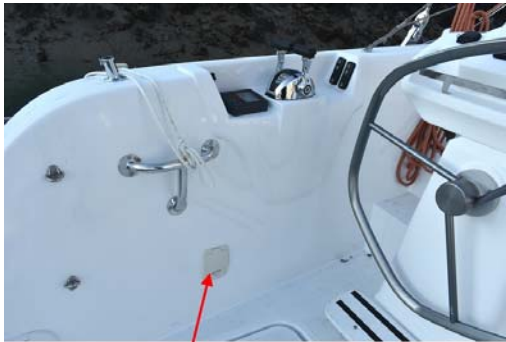
The manual bilge pump is in the cockpit.
