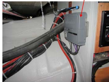
Vessel Management Unit Location: Port engine compartment
