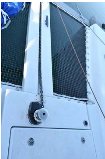
Electric windlass (sprocket diameter * 1 mm)
