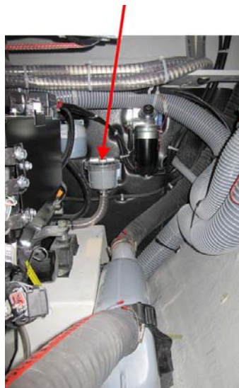
Seawater filter Location: Port engine compartment & Starboard engine compartment
