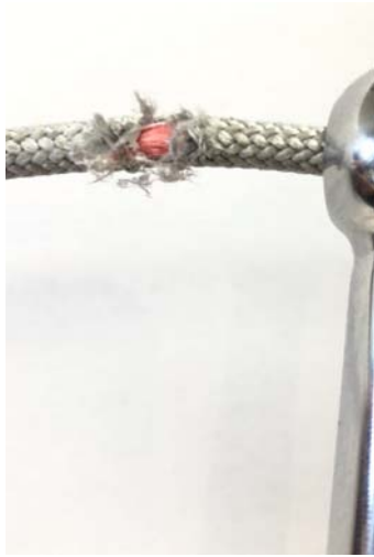
Example of fraying (the red core is visible)
