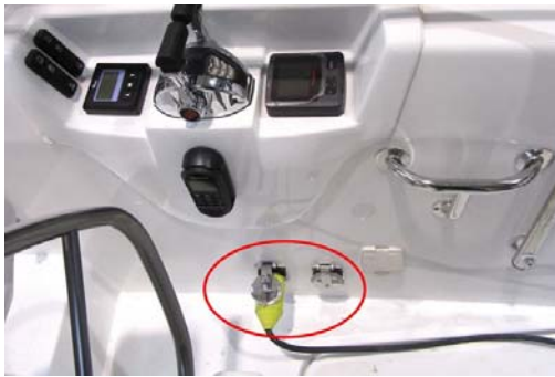
Ref 1: AC shore socket (onboard & Air conditioning) Location: Starboard cockpit
