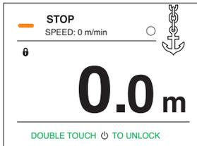
To unlock / lock the instrument quickly press ⏻ key twice.
